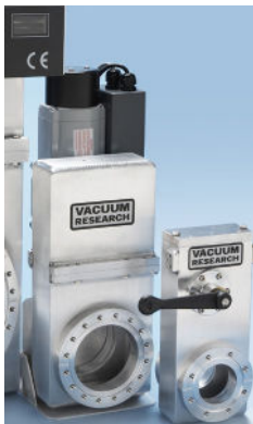
Stainless steel & aluminum valves with Conflat® flanges. Aluminum has less outgassing than stainless steel. Up to 2 orders of magnitude less, see references on page 39.
