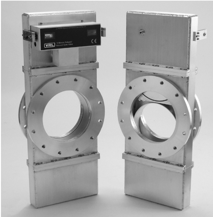
Valve on left is fully open with protective ring in place. Particles are directed through the port instead of into the valve body.
