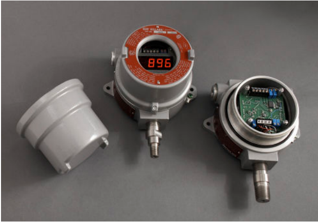
Sensor and gauge with & without optional digital display. Both provide 4 - 20 mA and 0-10 VDC output. Enclosures meet ATEX 95 equipment directive 94/9/EC requirements for Apparatus Group II, Categories 2G/2D: II 2 G EEx e II T3-T4; II 2 G EEx D IIC T3-T4; II 2 D IP66 TI 10°C - T140°C.
