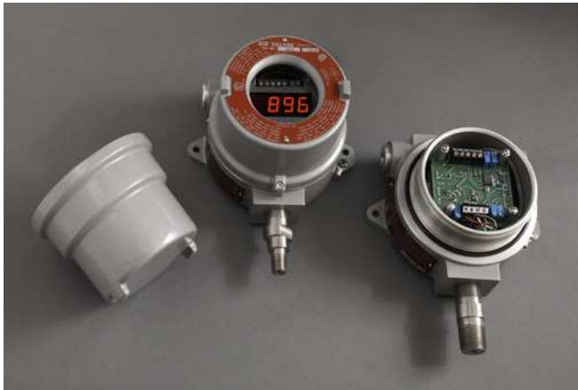
Sensor and gauge with & without optional digital display. Both provide 4 - 20 mA and 0-10 VDC output. Enclosures meet ATEX 95 equipment directive 94/9/EC requirements for Apparatus Group II, Categories 2G/2D: II 2 G EEx e II T3-T4; II 2 G EEx D IIC T3-T4; II 2 D IP66 T1 10°C - T140°C.
