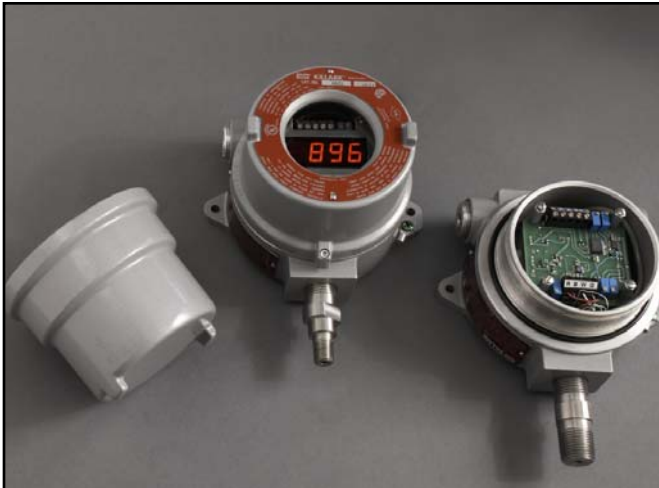
Sensor and gauge with & without optional digital display. Both provide 4 - 20 mA and 0-10 VDC output. Enclosures meet ATEX 95 equipment directive 94/9/EC requirements for Apparatus Group II, Categories 2G/2D: II 2 G EEx e II T3-T4; II 2 G EEx D IIC T3-T4; II 2 D IP66 TI 10°C - T140°C.
