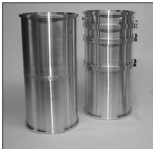
Modular vacuum chambers with ISO-320k flanges and lengths of 100, 200, 400 & 800 mm. Inside diameter is 362 mm.
