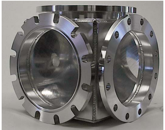
Aluminum cube with three, 10 inch ANSI flanges (11.7 inch ports) to join a cryo pump to two chambers.
