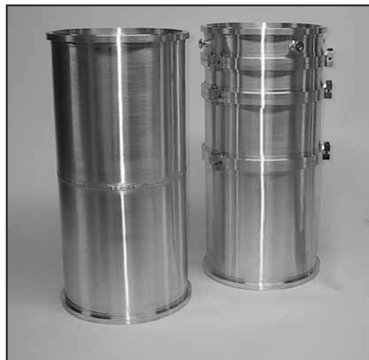
Modular vacuum chambers with ISO-320k flanges and lengths of 100, 200, 400 & 800 mm. Inside diameter is 362 mm.
