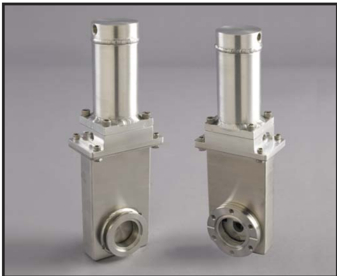
Valve on the left has NW-40 flange. Valve on the right has special 2.75 In. Conflat® flange. Standard practice is for bolt circle to straddle center line.
