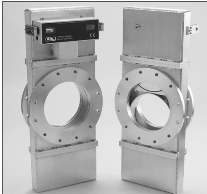
Valve on left is fully open with protective ring in place. Particles are directed through the port instead of into the valve body.
