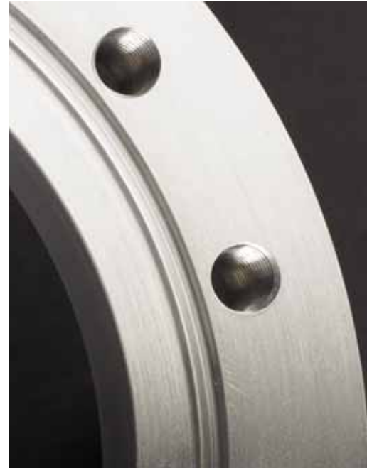
Aluminum CF Flange After 100 Closures
