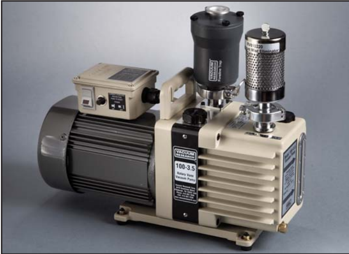
Photo shows Pump with optional inlet trap and exhaust mist eliminator installed. See page 16 to order these accessories. Power on/off switch, resettable circuit breaker and line cord are standard on pumps shipped with single phase motors.
