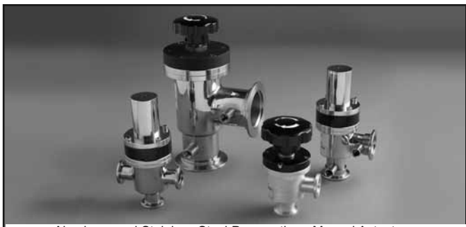
Aluminum and Stainless Steel Pneumatic or Manual Actuators, Angle or Inline Style with Port Sizes from NW-16 To NW-50
