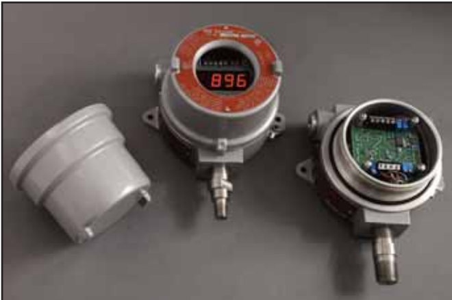
Sensor and gauge with & without optional digital display. Both provide 4 - 20 mA and 0-10 VDC output. Enclosures meet ATEX 95 equipment directive 94/9/EC requirements for Apparatus Group II, Categories 2G/2D: II 2 G EEx e II T3-T4; II 2 G EEx D IIC T3-T4; II 2 D IP66 TI 10°C - T140°C.
